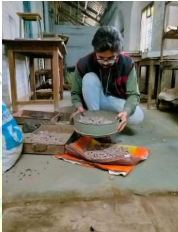
Figure 2. RAP Material (Filtration Process)
